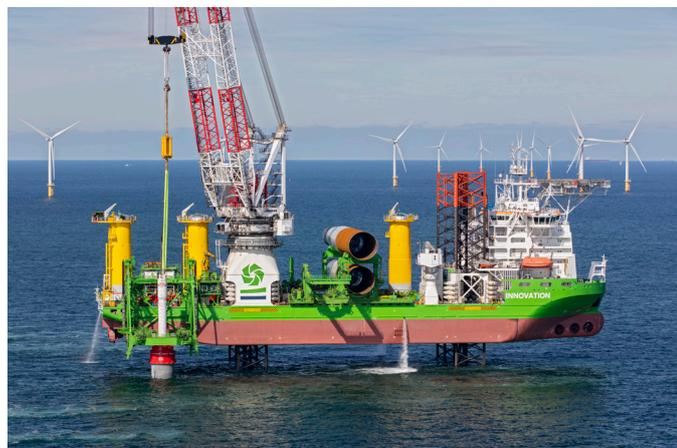
overall gripper weight down. The unique combination of gripper stiffness with the slenderness of the construction enabled DEME to maximize the useful payload on its jack-up. Our unique Pendulum Design increased the versatility and piling accuracy of HLJV Innovation.
