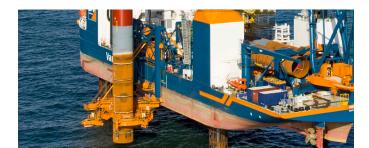
The good collaboration and installation results encouraged Van Oord to return to TWD with a request for a mirrored version of the gripper on jack-up vessel Wind Osprey. Both Aeolus and Wind Osprey were mobilized to install wind turbines on Gemini Offshore Wind Farm.
