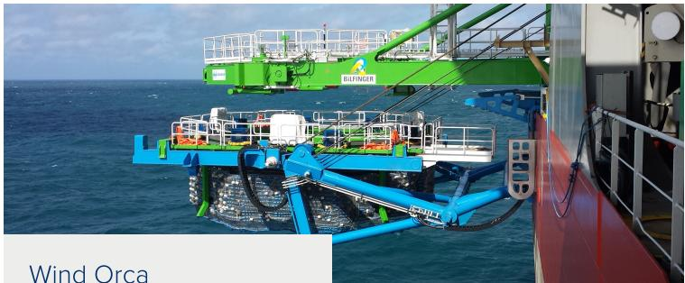
For the monopile foundation installation on the Sandbank Offshore Wind Farm project, Bilfinger rented Cadeler's jackup vessel Wind Orca. TWD was selected as an engineering partner to deliver the full services, from design (e.g., a monopile gripper, a hydro sound damper [HSD] deployment frame, an upending hinge, and various sea fastening structures) to fabrication supervision on Wind Orca.
